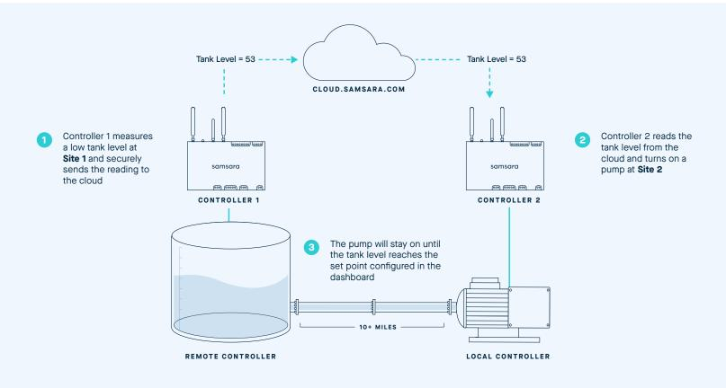
Remote Variables: Using remote variables, Central Texas can collect data points at one location and use them to control outputs at a second location.
